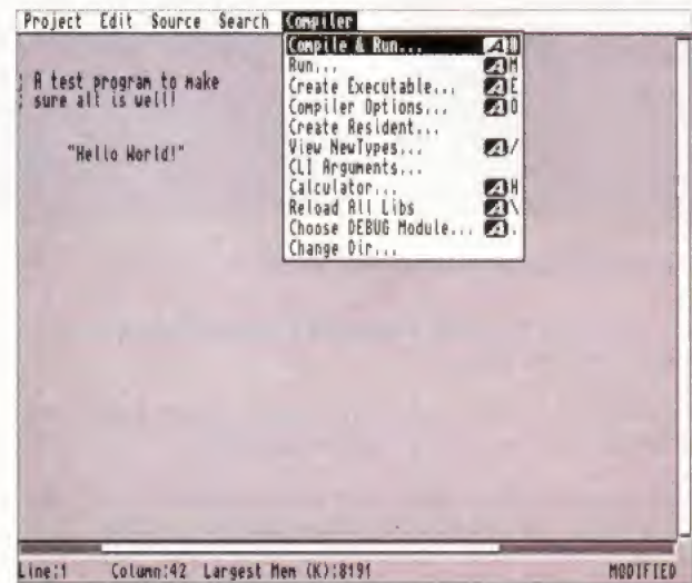
The "Compile & Run" menu option will compile your code into memory and then execute it.
